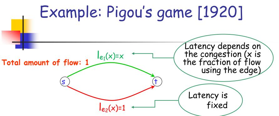
Is there any Nash flow for this game? YES! That in which all the flow travels on the upper edge ⇒ the cost of this flow is C(f) = 1·|<sub>e1</sub>(1) +0·|<sub>e2</sub>(0) = 1·1 +0·1 = 1
